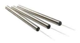
The HTFC Series fiber optic coupler is based on Agiltron's fused biconical taper technology and special packaging structure. It features good uniformity, low excess loss and very low polarization sensitivity. The device is ideal for splitting or combining light with exceptional performance over a wide wavelength range. 1310 or 1550nm are standard wavelength band, other wavelength band is available as special orders.
