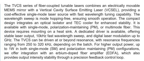
The device is highly ESD-sensitive to electrostatic discharge due to its thin active laser layer configuration; consequently, only the protected benchtop has a warranty.
