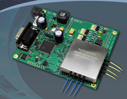
Leveraging Agiltron's advanced MEMs and fiberoptic technologies, Agiltron offers an exceptional range of all-optical switching systems over broad wavelength and variety of optical fiber (SM, PM, MM up to Imm core fiber).
